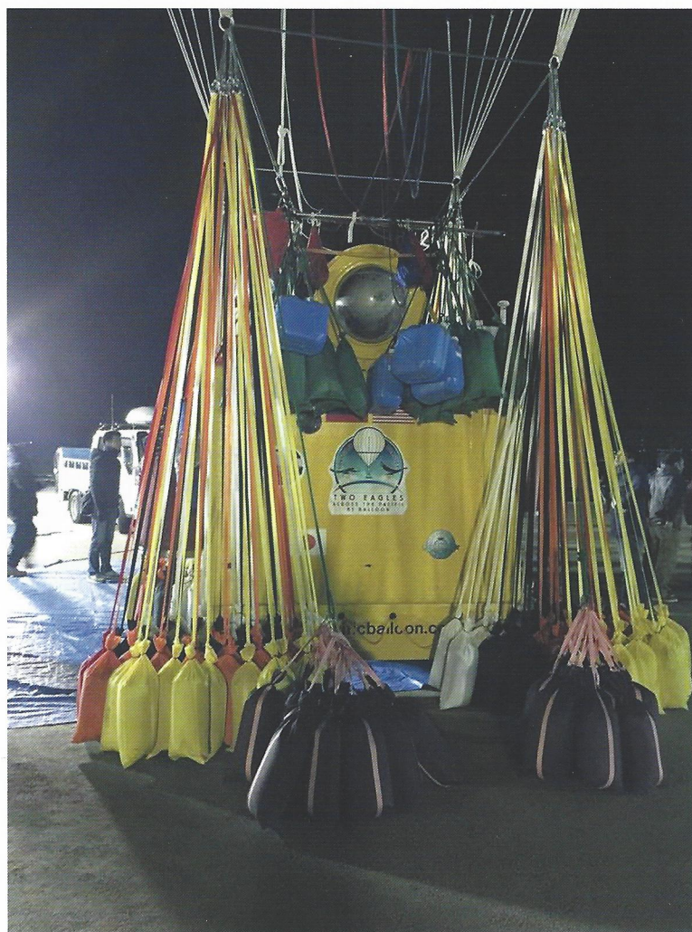
The Two Eagles gondola ready for launch. The colored ballast bags and ropes helped the pilots keep a running total of ballast expended and remaining.
