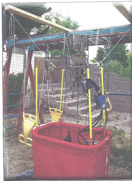
This backyard swing set rig served to allow Bobby to practice emergency burner relights and other skills ad nauseam.
